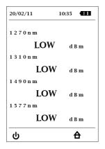
The instrument is now ready for measurements. Power levels of the respective wavelengths in live fibers will be displayed automatically when appropriately connected at OLN & OLT ports.
